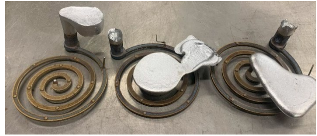
Figure 12. As-cast spirals in HAM from last poured (left) to first poured (right).
