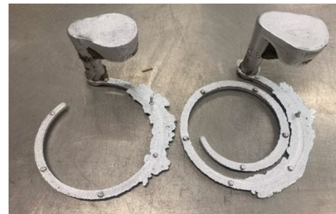
Figure 13. As-cast spirals in No-Bake from last poured (left) to first poured (right).
