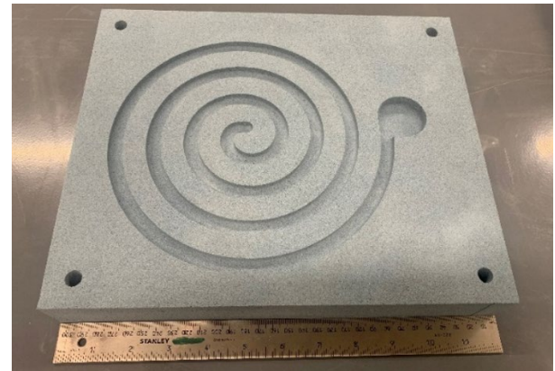
Figure 5. Machined modified non-standard fluidity spiral in HAM.
