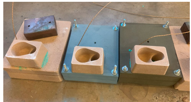
Figure 7. Assembled experimental molds shown with basins and thermocouples.
