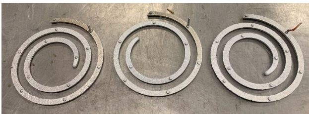
Figure 11. As-cast spirals in 3DP from last poured (left) to first poured (right).
